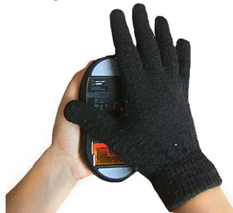
Figure 12: A glove served as a work around to overcome the limited focal range of our device.
