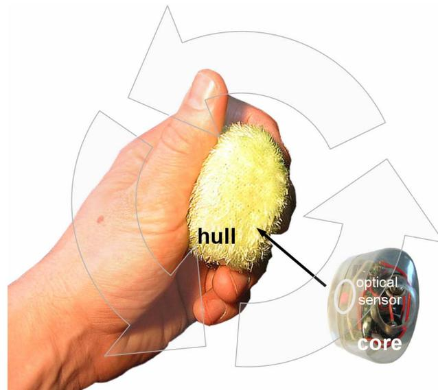
**figure 1:** The core of soap is an optical sensor. The core can rotate freely inside soap's elastic hull. While pointing, users cause soap's core to rotate by applying off-axis pressure. The relative motion between core and hull is picked up by the optical sensor inside the core.
