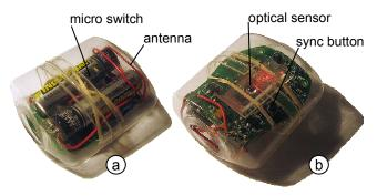
Figure 3: The soap core (a) top & (b) bottom view. A micro switch in a slightly elastic casing allows users to generate a click by squeezing the device.
