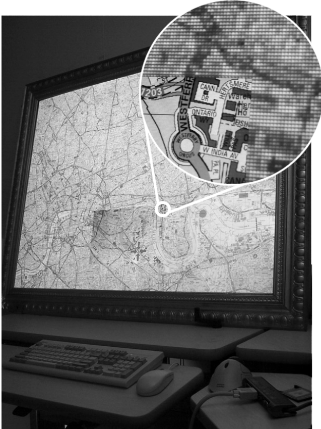
Figure 2: The high-res region in the center of this focus plus context screen provides users with detail information.
