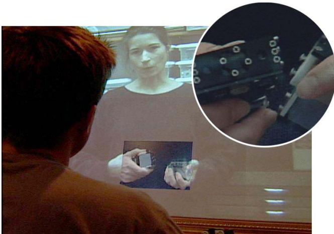
Figure 8: A videoconference partner displayed on an f+c screen. The higher resolution in the focus region allows communicating relevant details.
